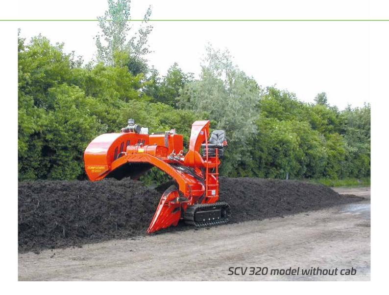
The lateral conveyors allow to improve turning and develop perfect windrow formation and cleaning of the sides.
