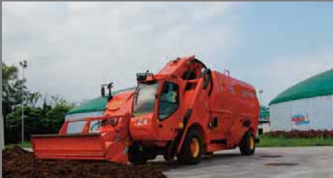
Self Turbo Refiner during loading, grinding and mixing of manure.
