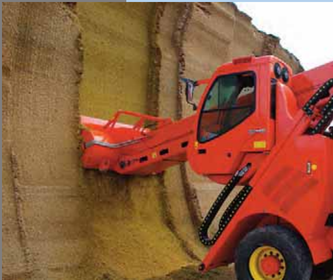
Self Turbo Refiner during loading, grinding and mixing of silage.
