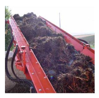
blades. During chopping, the products are also actively mixed, resulting in a homogenous shred ready for composting. The SAMURAI chopper can also perform other functions, such as: mixing compost with additive products or mixing sludge or digestate.
